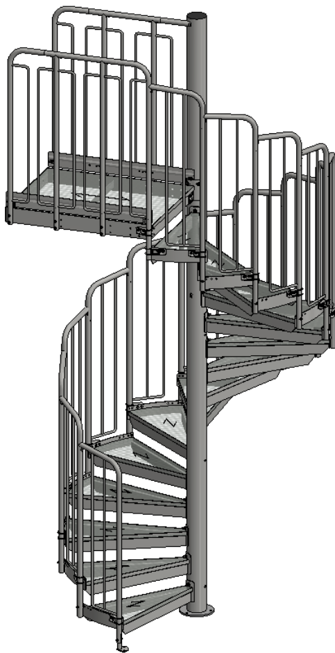
Figure 1. Landing with straight exit
