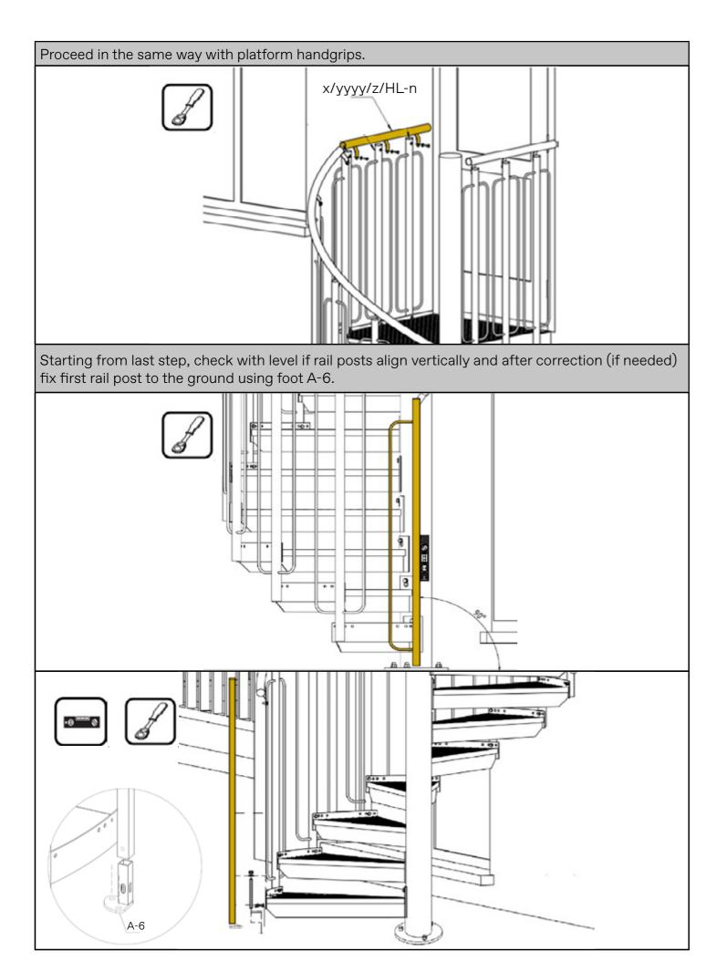
In the case of stairs with a radius greater than 1250 mm, the post no. 2 (R-2A) is fixed with an ad-ditional plate to fix to next step (using M8×25 bolt (D), 2 washers 8 (J) and a M8 nut (E) and to the ground with the foot M-D-A-6.
