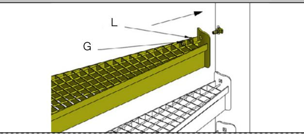
ALTERNATIVE METHOD – WITHOUT USING LOCKING WASHERS First insert hammer bolts (C) into square holes of step's fastening plate. Put M12 washers (L) and screw self-locking M12 nut (G) using fingers until it's possible (till the moment when end of bolt's thread reaches nylon insert in the nut).
