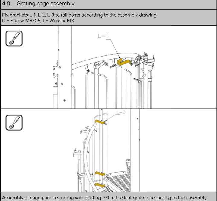
drawing. Use top parts of grating fixings (L). A – Bolt M10×50; M – grating fixing (top part) G-11; K – Washer 10; F – Nut M10
