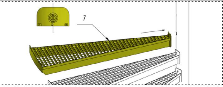
After inserting the hammer bolt into the sockets, turn the hammer bolts to the horizontal position and then move the whole unit towards the column base until it stops. Tighten the screw connection using approx. 60% of the nominal tightening torque for M12 which is 70 Nm. Repeat procedure for every step in stairflight.
