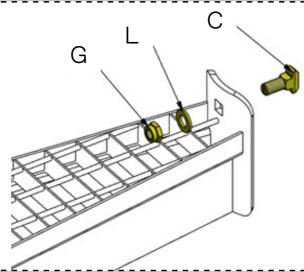
Set hammer bolts vertically - the position of the bolts is shown by the marker at the end of the bolt shaft. Attach steps by inserting the hammer bolts to the sockets in the central pipe.
